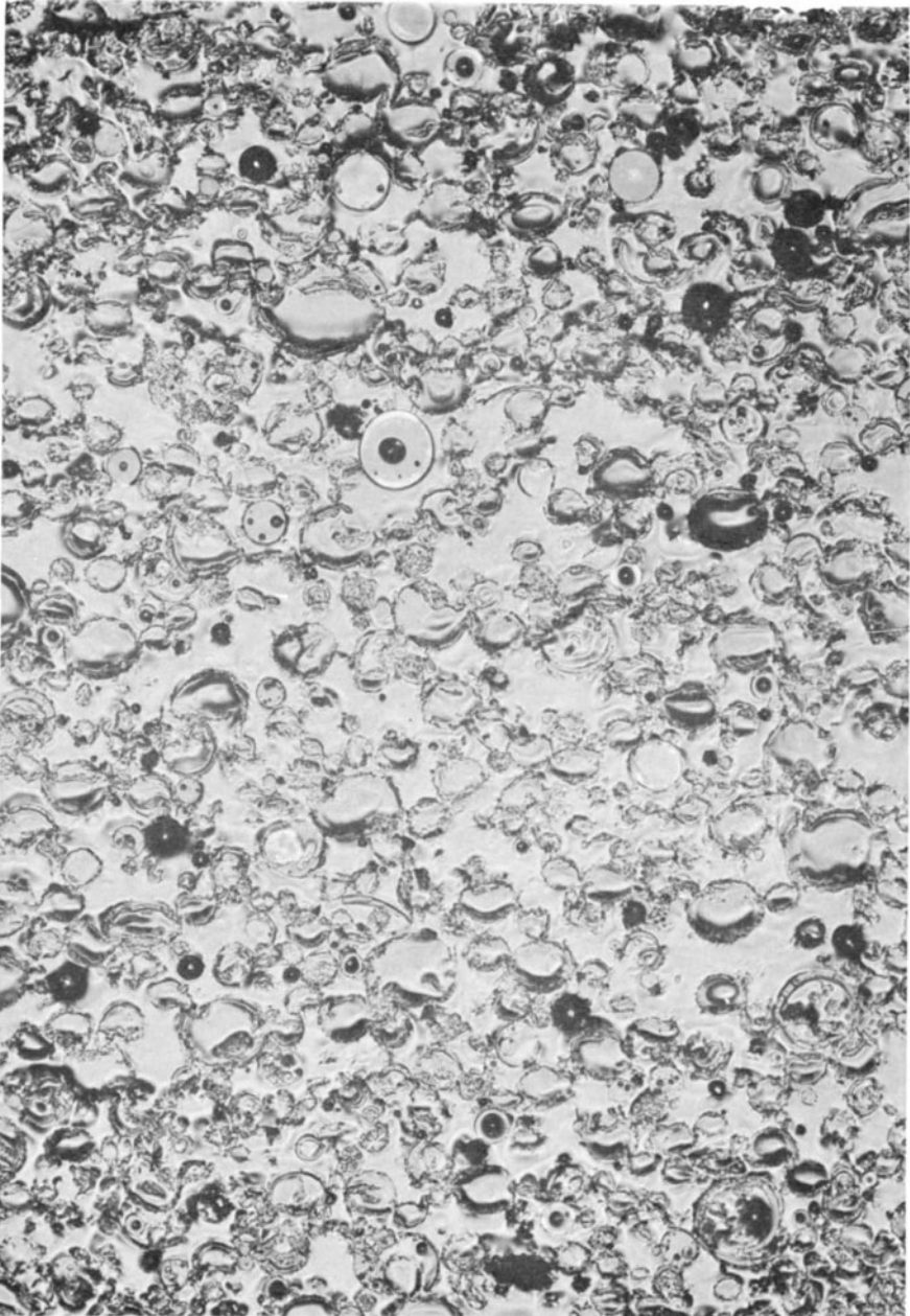
Fig. 3-3. Photomicrograph of syntactic foam after loading of 10 kilobars.
