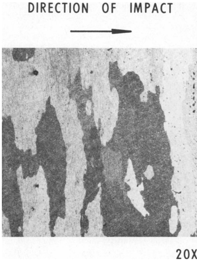
Fig. 2. Photomicrograph of the aluminum 1060-0 target material.
